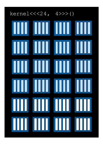
Depending on the number of SMs on a GPU, and the requirements of a block, more than one block can be scheduled on an SM
