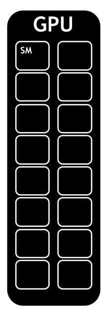
NVIDIA GPUs contain functional units called Streaming Multiprocessors, or SMs
