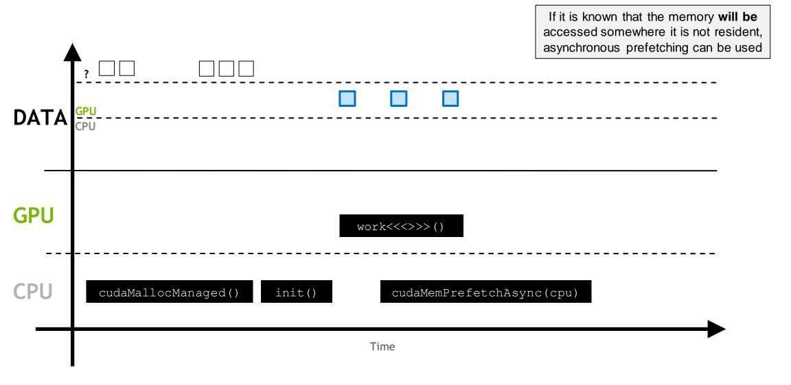
This moves the memory in larger batches, and prevents page faulting
