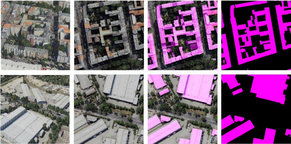
Figure 1: The concept of the aerial image simulation. We use 3D building models (left) as input, and simulate 2D aerial image, associated with many other attribute like building mask, building height, which can be used for uncertainty quantification of many downstream tasks.
