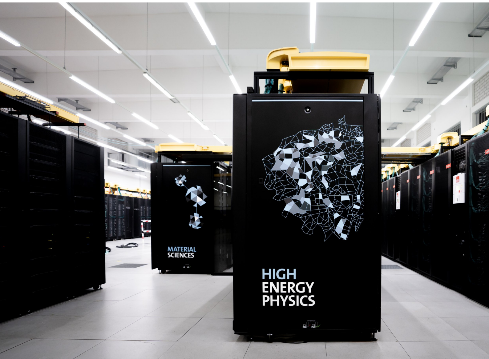
The high-performance computer SuperMUC-NG at the Leibniz Supercomputing Centre is based on Lenovo ThinkSystem SD650 DWC compute nodes and equipped with Intel Skylake Xeon Platinum 8174 processors. The machine hosts 6,336 thin compute nodes, each with 48 cores and 96 GB memory, and 144 fat compute nodes, each with 48 cores and 768 GB memory per node. User operation started in August 2019. (Picture: Axel König).
