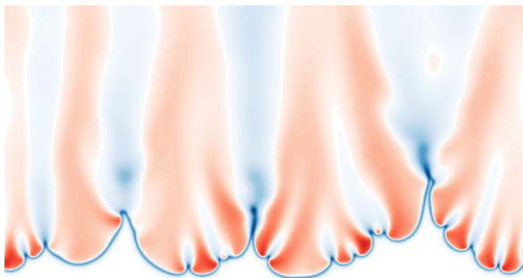
Figure 1: Snapshot of the temperature field showing small-scale cellular structures and large-scale finger-like structures along the flame front.
