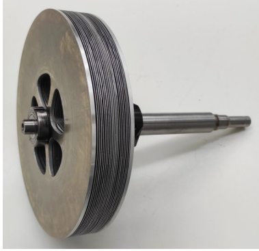
Figure 1: Sample Tesla turbine rotor with multiple disk gaps and outlet openings in the center.
