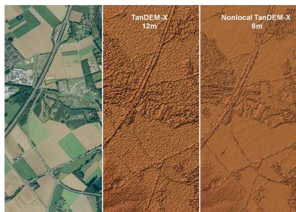
Figure 5: Jülich city area: Optical image ©Google (left), the standard 12m TanDEM-X DEM (middle) and improved nonlocal TanDEM-X DEM with 6m resolution (right) [7].
