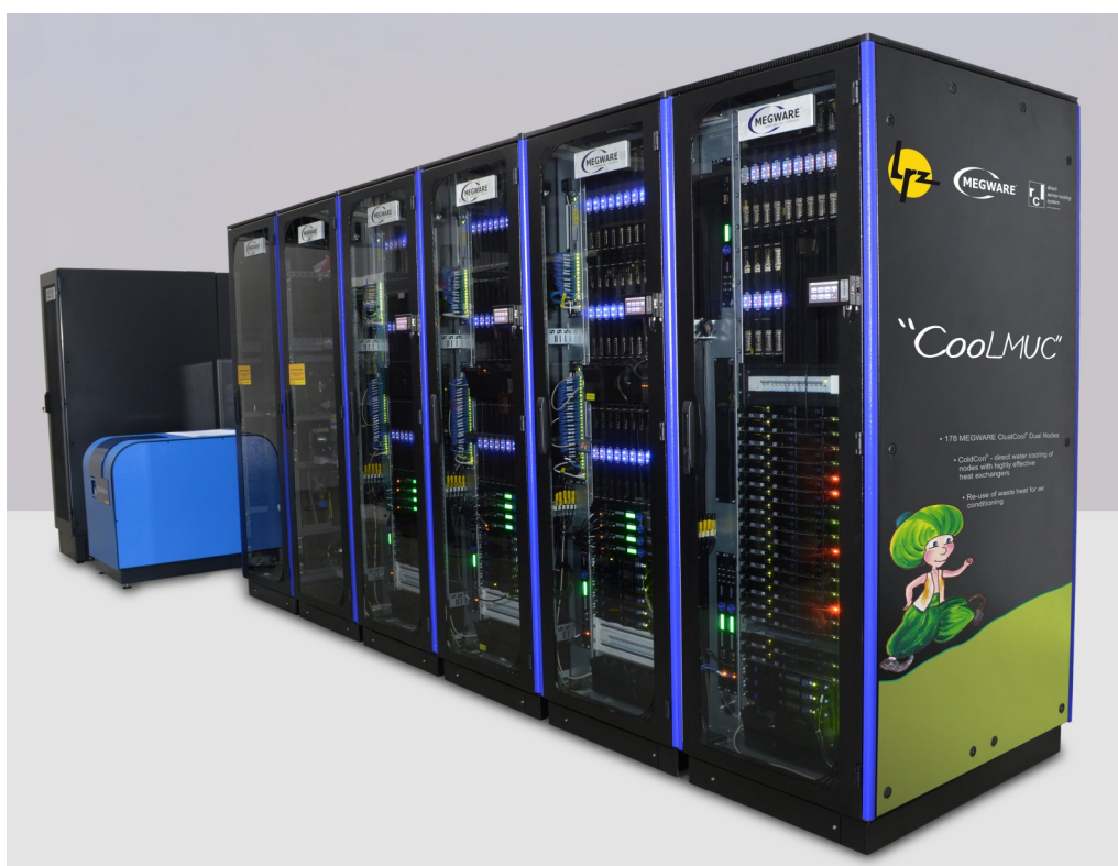
Figure 1: CoolMUC-1 (front) and adsorption chiller (back). Picture: Megware, CC-BY-SA 4.0.
