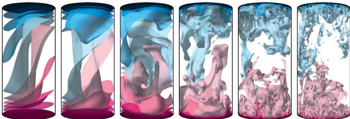
Figure 1: Instantaneous temperature fields in the non-rotating case. Shown are isosurfaces for ten equidistantly distributed values between the top and bottom temperature, blue corresponds to temperatures below the arithmetic mean temperature and pink to temperatures above it. The Rayleigh number increases from left to right from 10^5 to 10^{10} .
