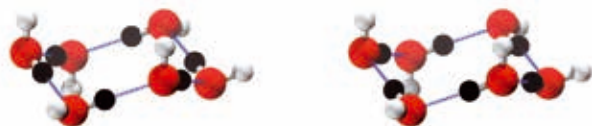
Figure 1: Schematic initial (left) and final (right) state of the transfer of six protons (black) in the proton-ordered six-ring (O: red; H: white; hydrogen bond: blue).
