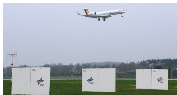
Figure 4: Flight experiments at Oberpfaffenhofen airport, confirming the efficiency of plate lines.
