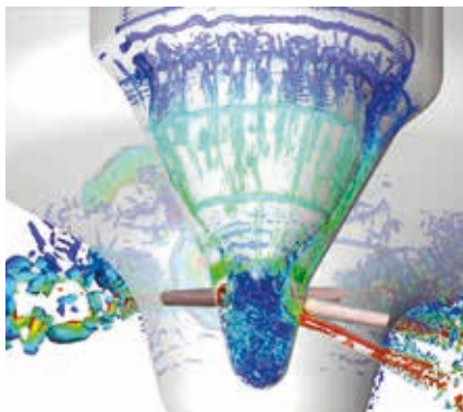
Figure 3: Coherent vortical structures during the main injection phase colored by velocity in the half-domain.
