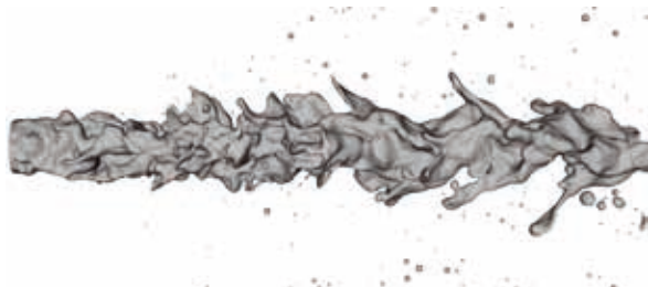
Figure 1: Gas-liquid surface of a spatially developing round jet with Re=5,000 and We=2,000 .
