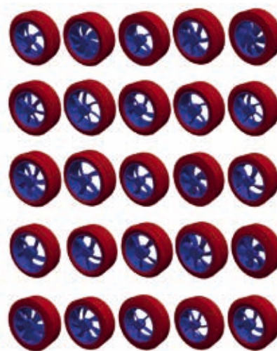
Figure 3. Fully Parametric Wheel based on DoE plan.
