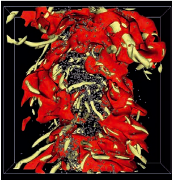
Figure 1: Spray combustion in TEJ; the gray spheres represent the liquid droplets (size is multiplied by factor of 5 for visualization), the yellow iso-surface is the Q-criterion showing the main turbulent structures, and the red iso-surface represents the temperature ( T = 1800 K)
