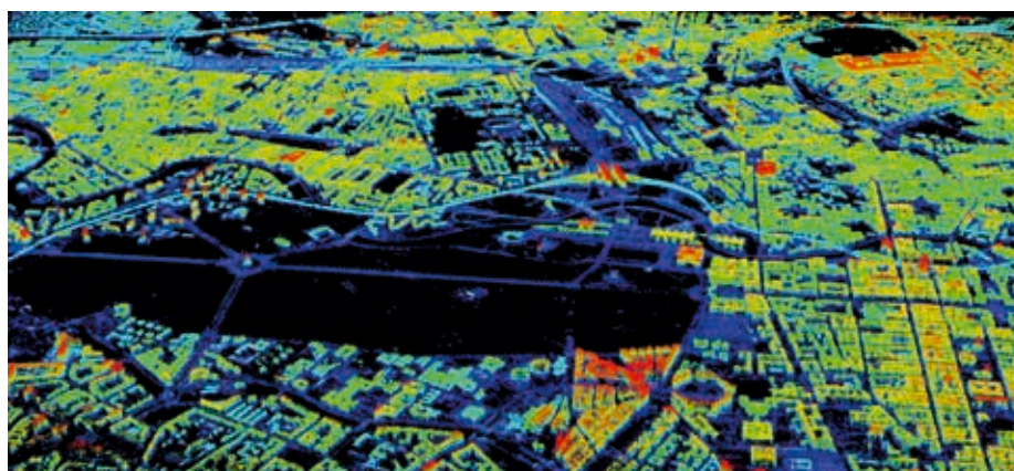
Figure 4: Fusion of two reconstructed 3D point clouds. The combined point cloud contains over 40 million points [5], [6].
