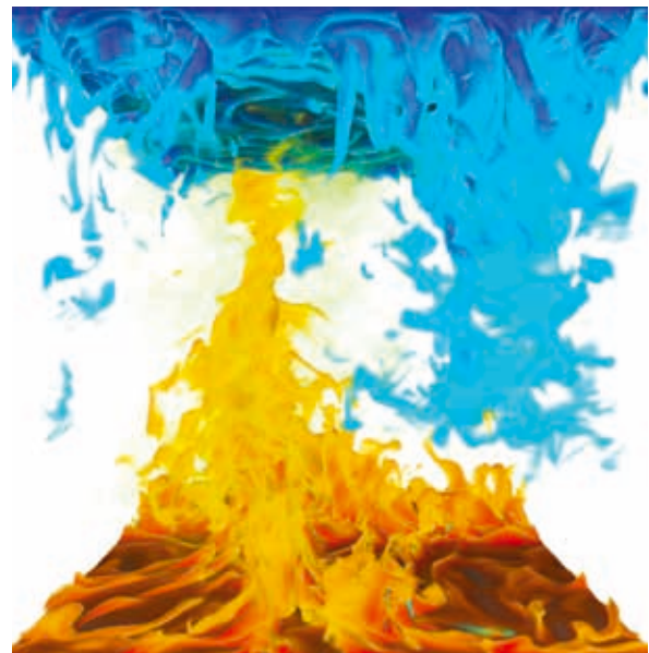
Figure 1: Three-dimensional visualization of Rayleigh-Bénard convection in a small periodic domain revealing the large-scale flow organization of a region with warm upwelling fluid represented in red and cold downgoing fluid in blue.
