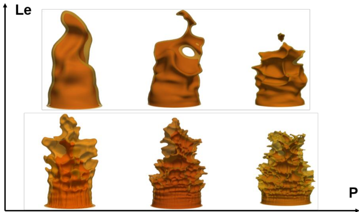
Figure 1: Turbulent premixed Bunsen flames (top) Lewis number Le = 1 and (bottom) Le = 0.34 at different pressure levels: 1 bar, 5 bar, 10 bar (left to right). The different colours represent different values of reaction progress variable.
