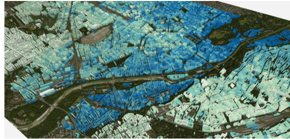
Figure 2: LOD1 city model reconstructed from the point cloud shown in Figure 1. Color from blue to white indicates height from low to high.
