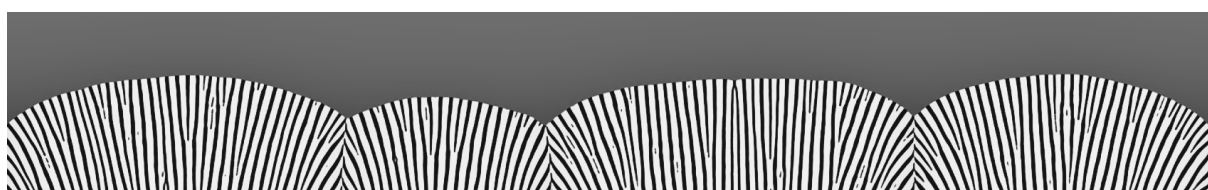
Figure 1: Exemplary solidification front of a simulated eutectic colony structure of NiAl-34Cr .
