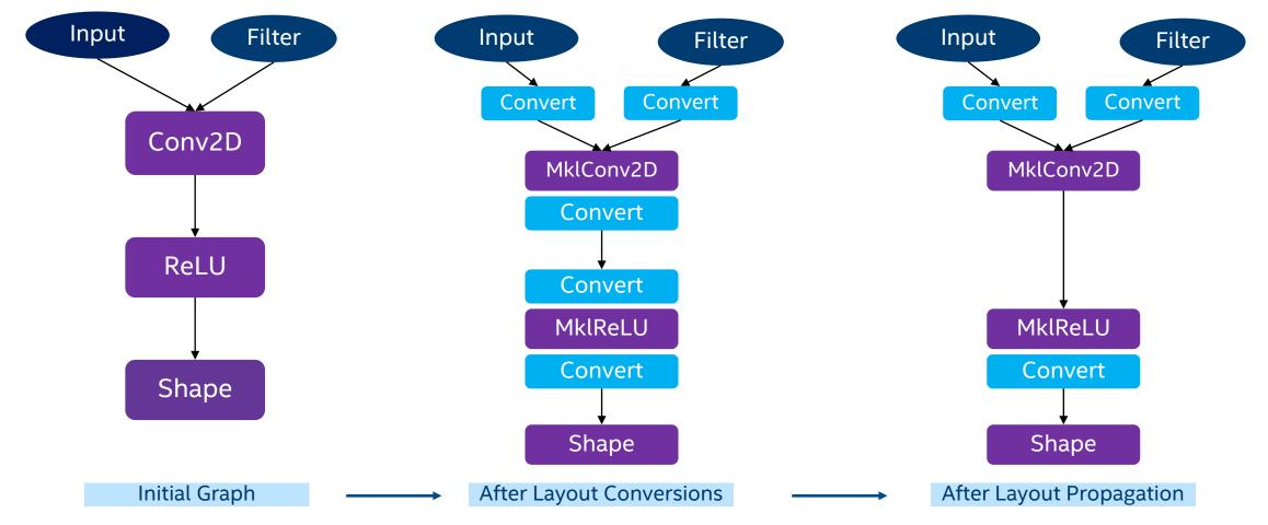
All oneDNN operators use highly-optimized layouts for TensorFlow tensors.
