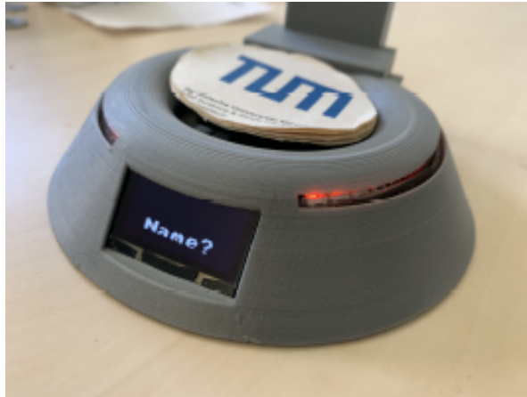
Figure 2.3.: The weight-based drinking detection device
