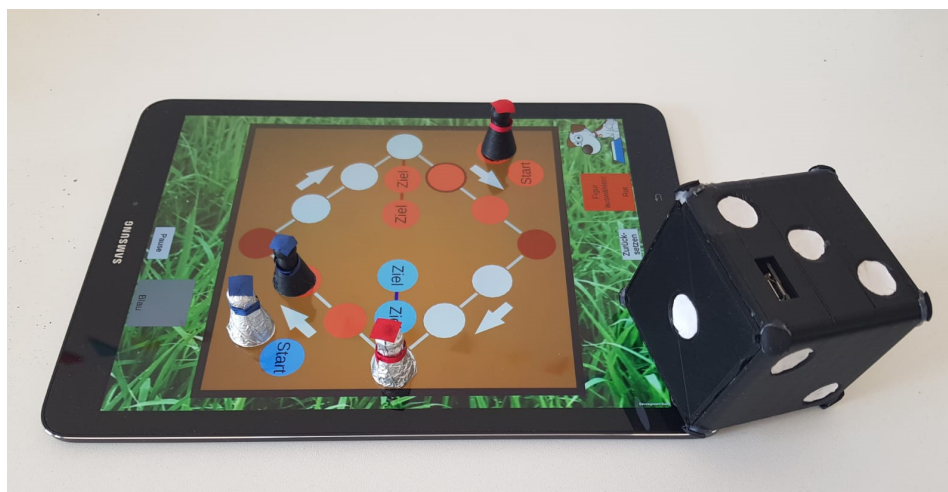
Figure 3.3.: The application, deployed on a tablet, with the developed pieces and the Bluetooth dice
