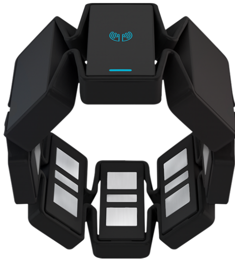
Figure 2.3.: Picture of the Myo[12].
