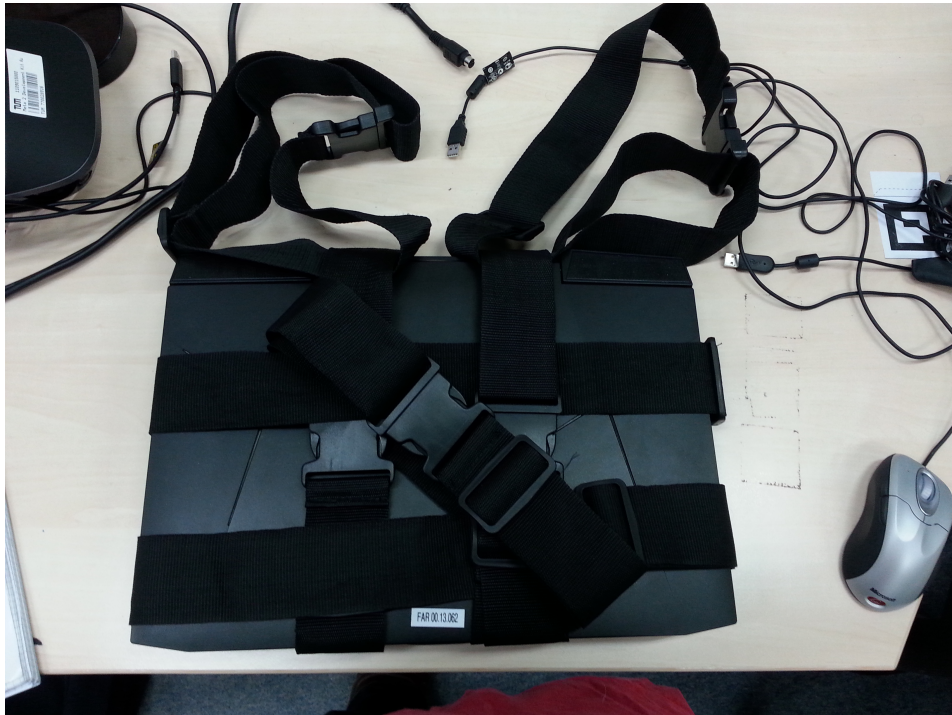
Figure 4.7.: Laptop strapped to be worn.
