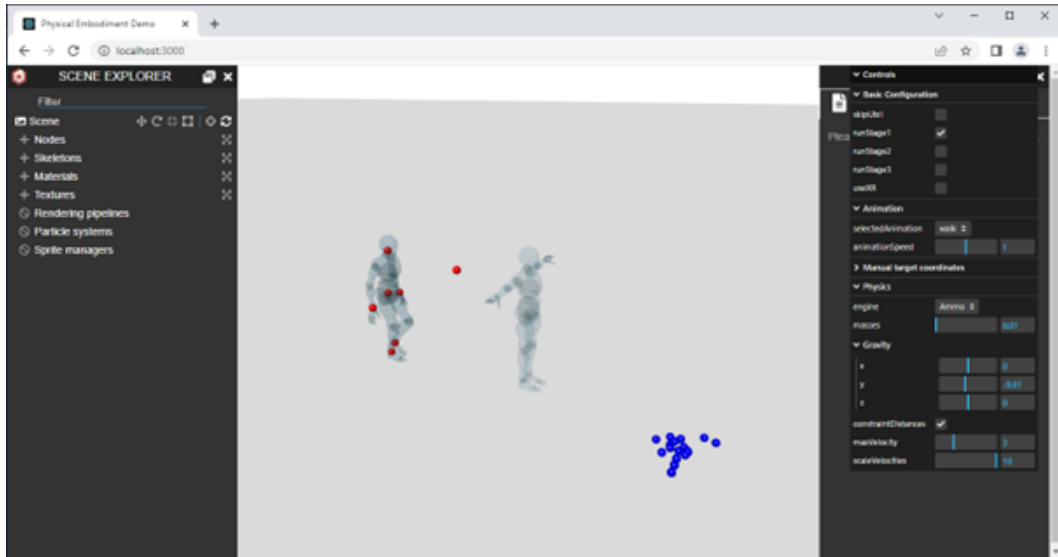
Figure B.1.: Screenshot of the web implementation. Only stage 1 is enabled, the other two stage avatars are in a unused state. The debugging UI on the right was used to make this configuration, along with enabling constraintDistances , which has no effect due to the disabled stage 3. The Scene Explorer on the left was kept in the application to allow examining the skeleton's structure.
