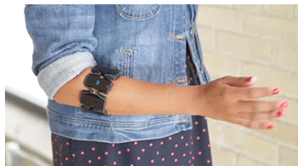
Figure 1: A person wearing the Myo armband correctly. It should be worn on the thickest part of the forearm [10].
