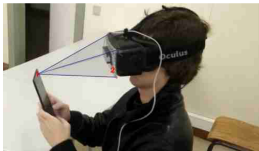
(a) The front camera of the smartphone tracks the marker on the HMD. Source: [10, Figure 3]
