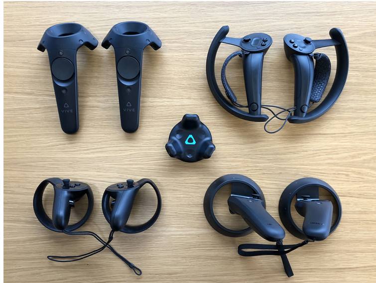
Figure 1.1.1.: A collection of different VR controllers. From left to right, top to bottom: HTC VIVE Controllers, Valve Index Controllers (“Knuckles”), VIVE Tracker, Oculus Touch Controllers, Samsung Odyssey Controllers. Source: [2]
