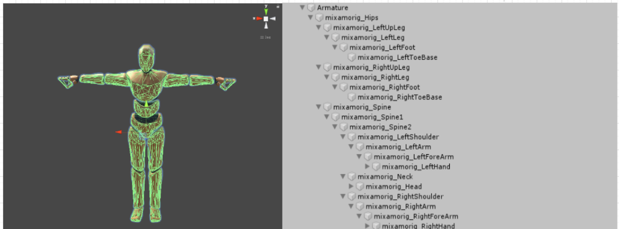
Figure 3.1.: On the left: The 3d model of a humanoid shaped avatar. The green areas are the surfaces that can collide. On the right: The hierarchical bone structure. All of these bones make a GameObject in Unity, with it's own position and rotation.
