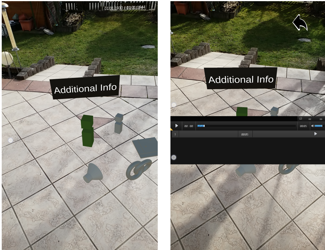
Figure 4.10: New 3D icons have been added to select the newly implemented scenes (left). The 3D speaker icon opens the audio player scene (right) which opens a player to play-back the audio file that can be uploaded in the Stolperstein form.
