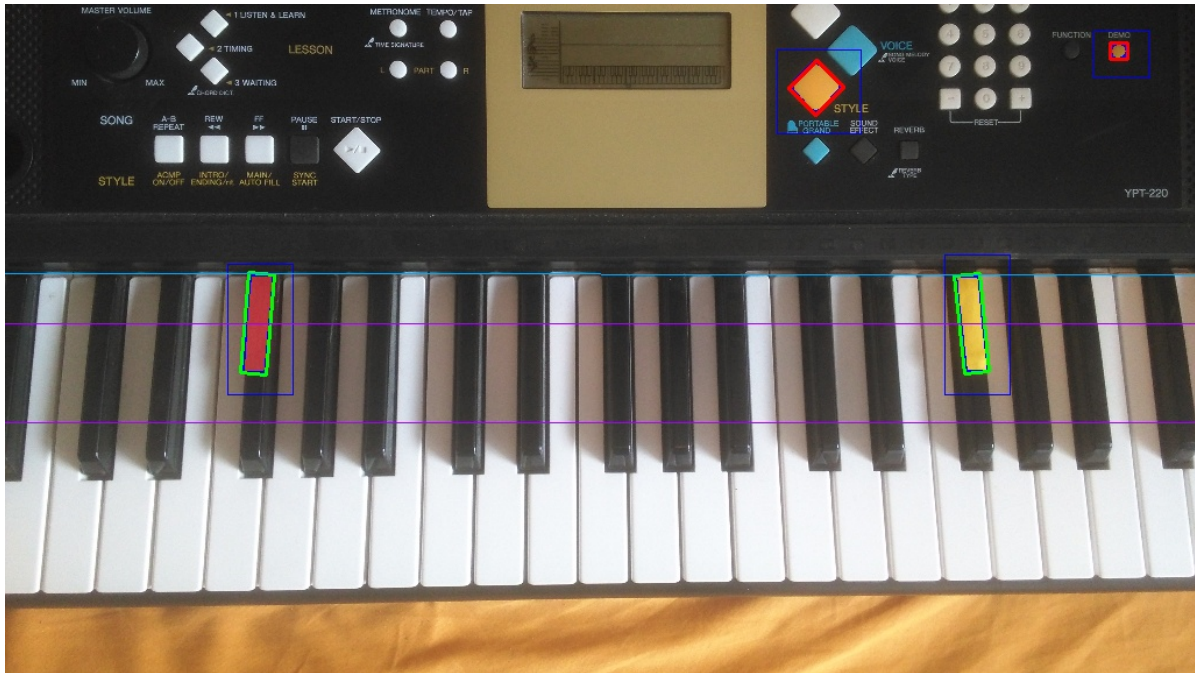
Figure 4.3: Output of the Marker Detection and Derived Information
