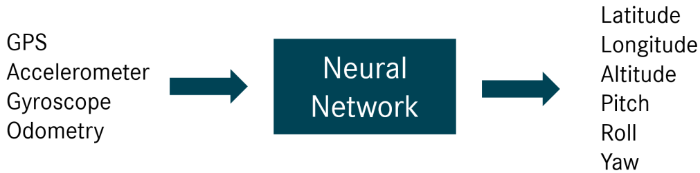
Figure 1.2: Schematic view of the approach to be developed. The input of the algorithm are different sensor measurements. The goal is to train a neural network which predicts a 6D pose estimate.
