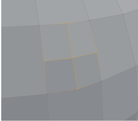
Figure 2.5: To subdivide individual faces on the UV-sphere, the faces are split vertically and horizontally and the new vertices have to be moved to sphere's surface according to the subdivision rules
