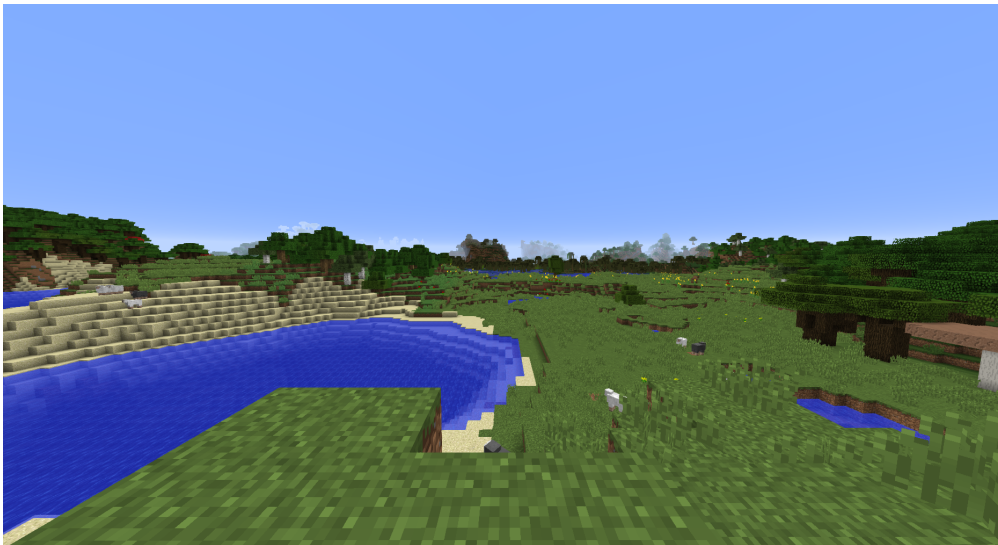
Figure 1.12: The world in MineCraft is made of blocks in a 3d grid. The noise function is evaluated at many grid cells and depending on the value a block or air is placed. The blocks between the evaluation points are linearly interpolated
