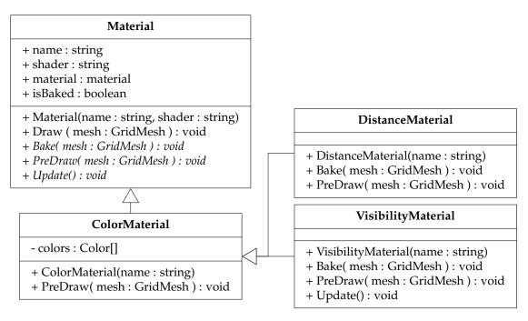
Figure 3.3: Class structure of selected GridMesh materials
