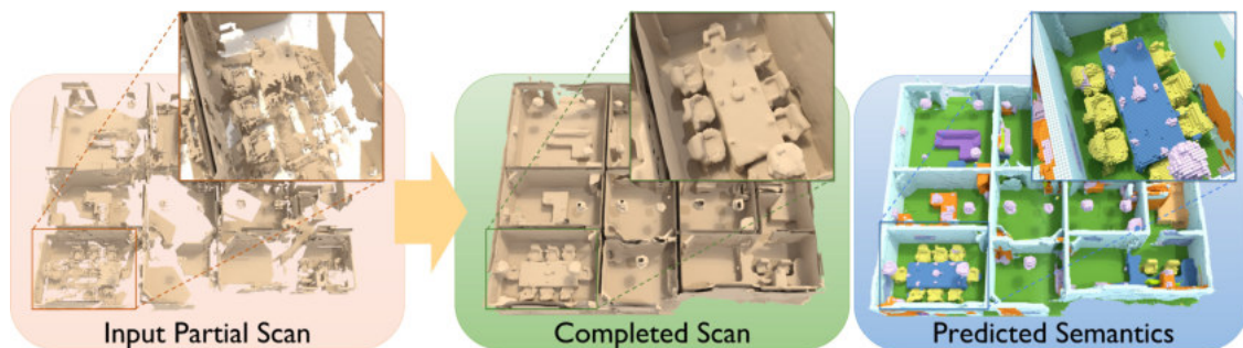
Figure 1.4.: Predicting the room semantics as proposed by Dai et al. First, they take the partial input scan and complete it through processing it in a specialised 3D CNN in different voxel resolutions. By doing this several times, they get a more precise prediction for the final room resolution, which is shown in the voxelized representation on the right. Image taken from [Dai, 2018].
