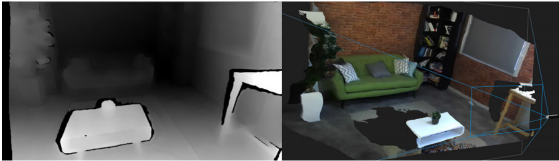
Figure 2.8.: Depth image generated with the stereo cameras from the ZED Mini. The left shows the recorded depth image, while the right showcases the resulting 3D point cloud. Areas that are obscured through other objects occlude entities and surfaces behind them, generating incomplete structures. Images taken from [Stereolabs, 2020b].
