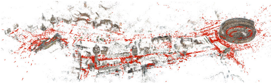
Figure 2.6.: A sparse point cloud of parts of Rome, created with SfM. This technique is able to recreate buildings from a collection of images based on found features across the set of samples. Image taken from [Schonberger, 2016].
