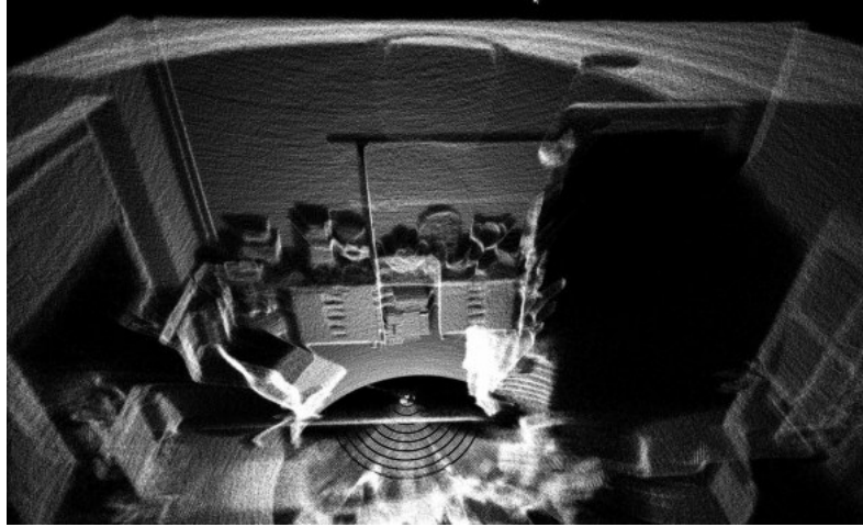
Figure 2.5.: A LiDAR scan of a room. This point cloud with almost five million points represents many details of the room, but some areas might not be reached with the scan and will create black holes within the point cloud. Image taken from [Hackster, 2017].
