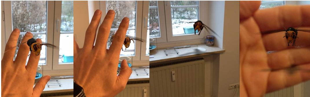
Figure 4.7.: Left images taken with the Iphone 12, the AR Object can be in the background, even so it gets clumpy sometimes. The right images, captured with the Pixel 3 don't support this function and the object moves to the foreground.
