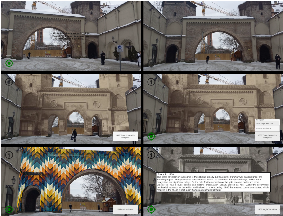
Figure 5.5.: Application Process. (Top Left) App started and a hint is displayed, (Top Right) after pressing the green button the localization process starts, (Middle Left) AR content is successfully overlaid, (Middle Right) from the menu in the right corner different stories can be selected, (Bottom Left) A different story is selected and the user moved, (Bottom right) another story is selected and after the info button, top left corner, is pressed a text the infotext is displayed.
