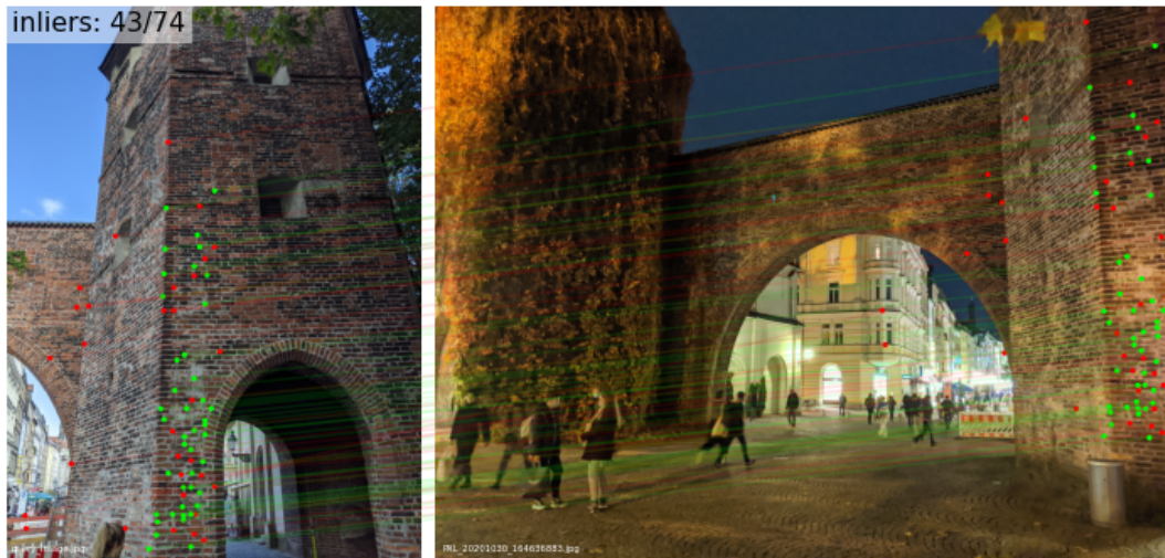
Figure 2.10.: Matching example. Inliners are points that fit the data model. This image shows 43 inliners (green) and 31 outliers (red). In this case false camera intrinsics were the cause for the high number of outliers.
