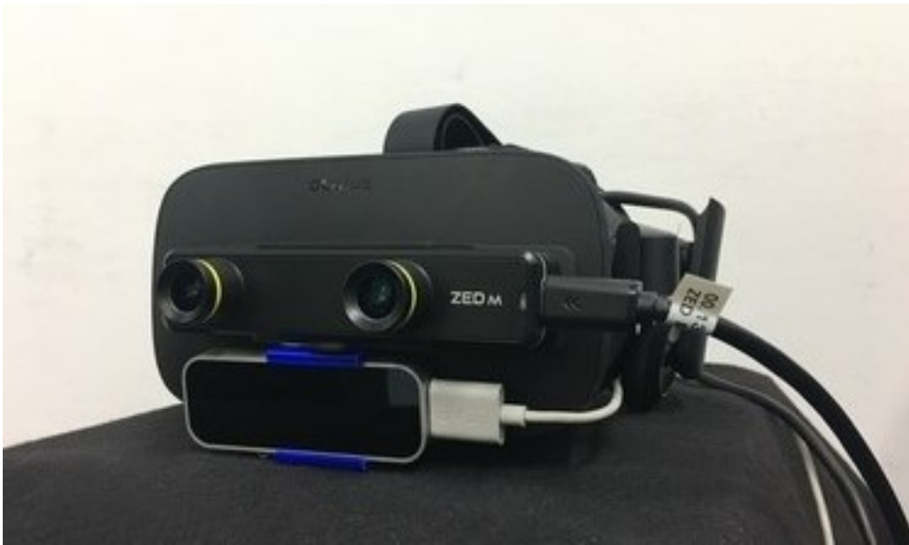
Figure 3.3: ZED Mini and LEAP Motion mounted on a Oculus Rift Source: Mehmet Dereli
