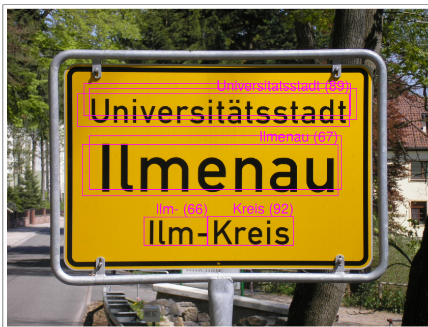
FIGURE 3.11: EAST preprocessing on sign photograph, decreased non-maximum suppression
