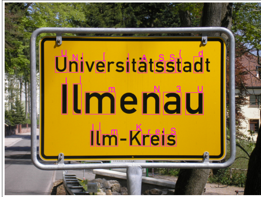
FIGURE 3.7: MSER preprocessing parameter adjustments on sign photograph
