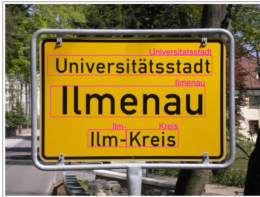
FIGURE 3.12: EAST preprocessing on sign photograph, decreased non-maximum suppression, decreased min confidence
