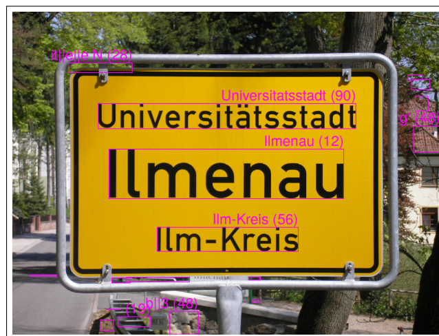
FIGURE 3.9: Pure Tesseract processing on sign photograph in “sparse” segmentation mode
