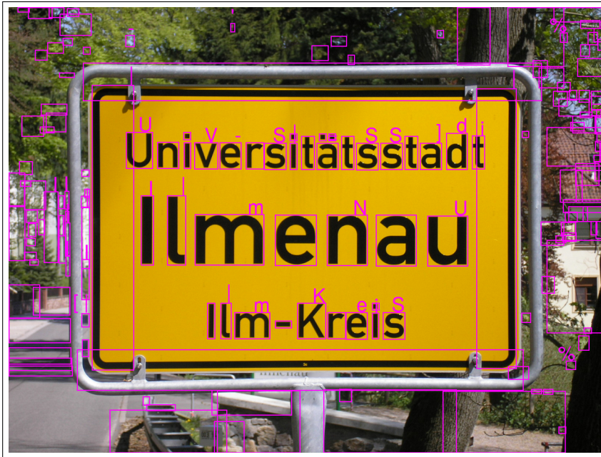
FIGURE 3.6: MSER preprocessing on sign photograph
