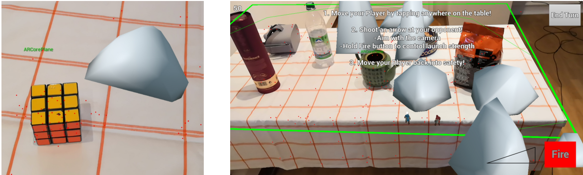
Figure 5.3.: Examples for the real and virtual world being misaligned after AR tracking was lost for a short amount of time.
