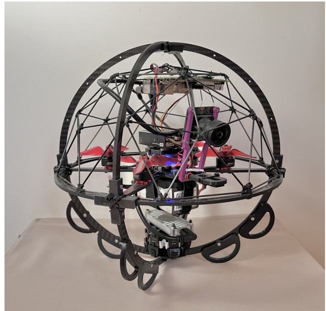
Figure 1: Indoor autonomously flying quadcopter Golden Snitch ensures Superhuman Sports Game a safe and tangible AR experience.
