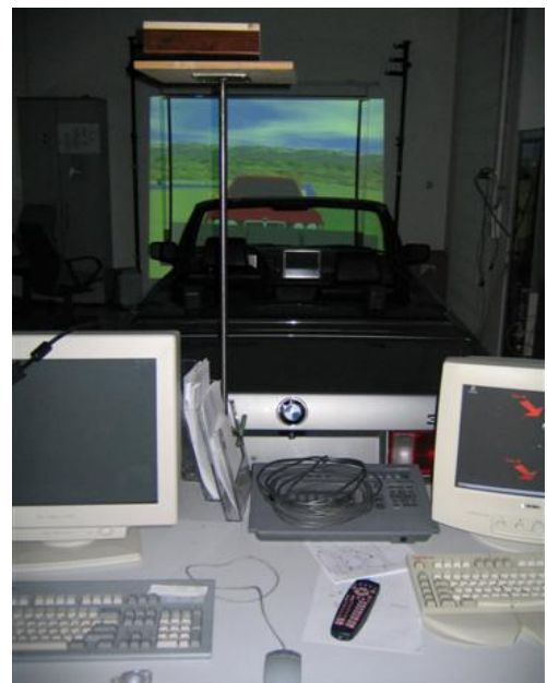
Figure 53: A view from the control desk showing the real car and the projected virtual world
