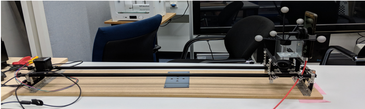
(a) Slider rail with stepper motor and mounted smartphone at the front
