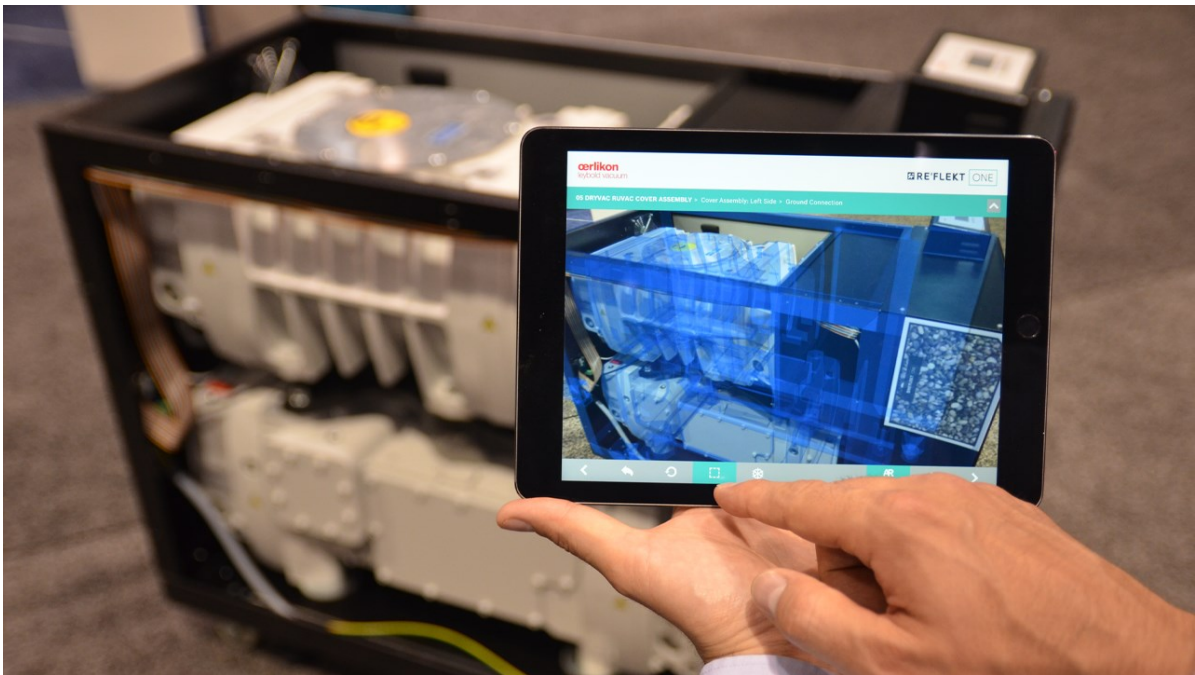
Figure 3.4: RE'FLEKT ONE being used on an iPad for an assembly procedure. Source: [83]
