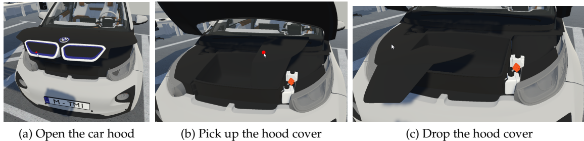
Figure 6.6.: Locating the emergency disconnect switch
