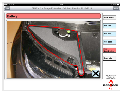
(a) Locating the 12V car battery
