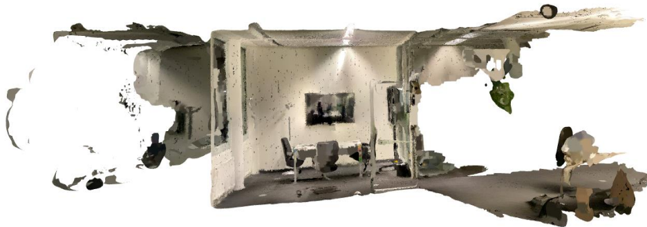
Reconstruction of a Point Cloud as a Mesh
