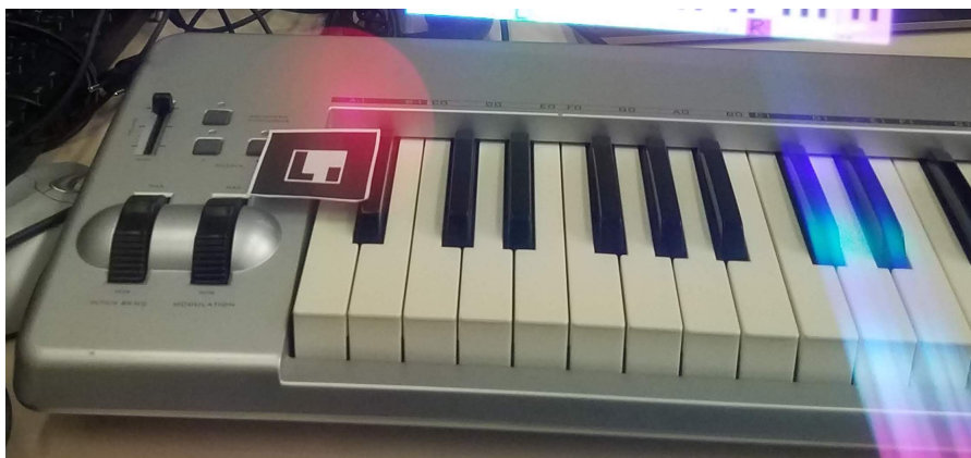
Figure 3.3.: Calibration: The red ball around the marker indicates that the marker has been detected
