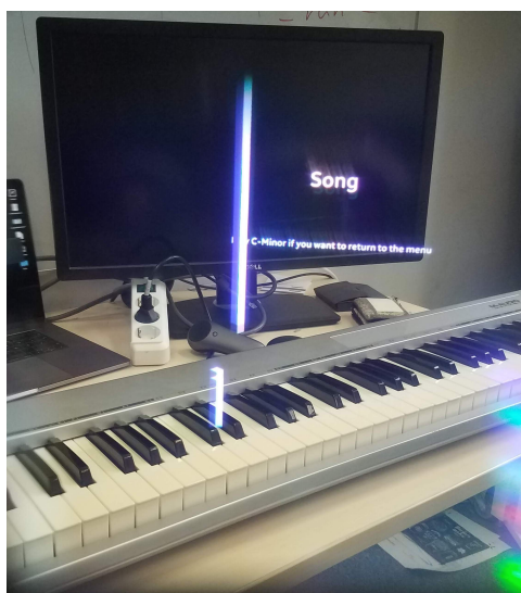
Figure 3.7.: "Hero" mode: The white box indicates a note that has to be played as soon as it hits the key
