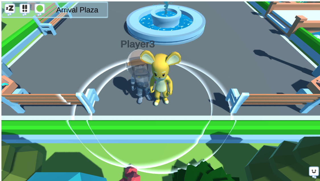
Figure 4.16.: If another avatar gets too close to the user, the avatar will be hidden partly to prevent model overlap, visual clutter and protect private space. In this case, Player3 will still see their character, while the yellow character is transparent instead. Source: Virtual Campus App
