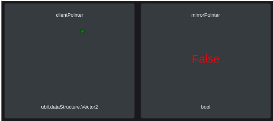
Figure 5.4: This pictures shows the cards used as message inspectors. In the left a green dot represents coordinates. In the right a boolean is printed.
