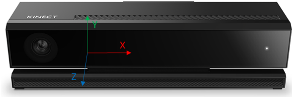
Figure 4.1: Kinect V2 and the positioning of the camera space coordinate system [17]
