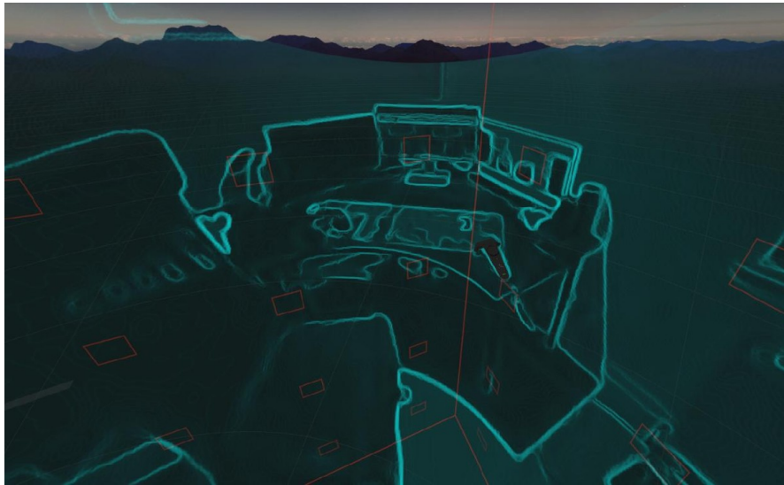
Figure 1.2: The chaperone system of the HTC Vive showing a boundary and outlines of real objects [Bro17]
