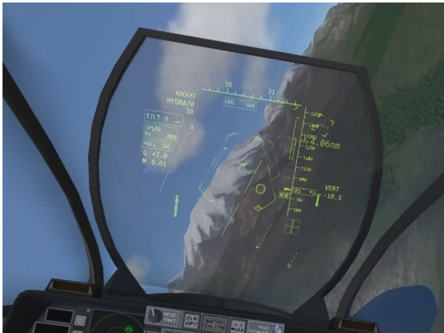
Figure 5.13: A screenshot from the game VTOL VR which shows the virtual horizon indicator aligned with the horizon in the middle of the planes head-up-display [BV18].
