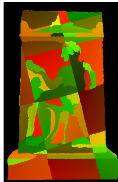
Figure 4: This image shows the stele with its texture coordinates visible. The coordinates are encoded in the red and green values of this image. Each of them corresponds with a pixel on the object's texture.
