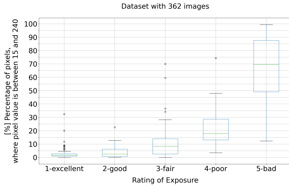
Figure 6.4: Boxplot over the percentage of dark and bright areas from the images from Test Dataset (chapter 5.3).
