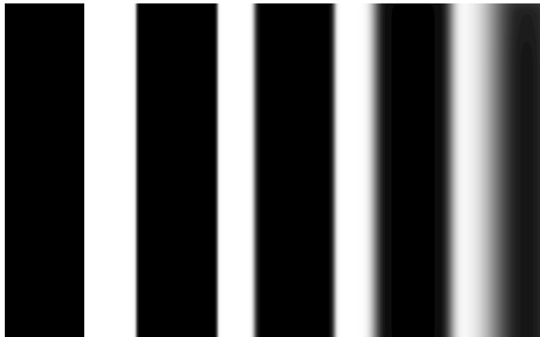
Figure 3.1: Here are five columns with transitions of different thickness at the edges. From left to right the sharpness decreases noticeably.
