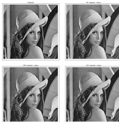
Figure 2.4: Original as well as compressions of Lenna image, with ranks 60, 100 and 120. The image demonstrates that an approximation with rank 100 is sufficient for most applications 1 .
