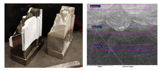
Example of the hybrid part, where base part was manufactured by subtractive manufacturing from H13 steel, and the top having complex inner cooling channels, was additive manufactured using maraging steel. The illustrated interface is dense and homogeneous.
