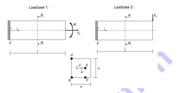
The shown clamped beam of length *I* is subjected to the moment *M* about the *y*-axis and the normal force  $F_1$  at it's free end in loadcase 1 and to the force  $F_2$  in loadcase 2. The cross-section and the modulus of elasticity are constant along the beam's x-axis. Each subtask is referring to only one of both loadcases. Use the given coordinate system with its origin in the cross sections centroid *C*.
