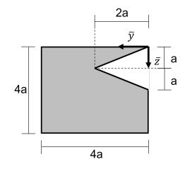
Shown is the cross section of a beam with measurement a. **Given:** a,  $(\bar{y}, \bar{z})$ -coordinate-system
