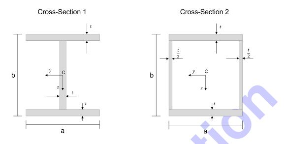
For the shown cross sections, which statement is true? ( $I_{yy}$  and  $I_{zz}$  are second moment of areas about the respective axis and  $I_T$  is the torsion constant of the cross-section)
