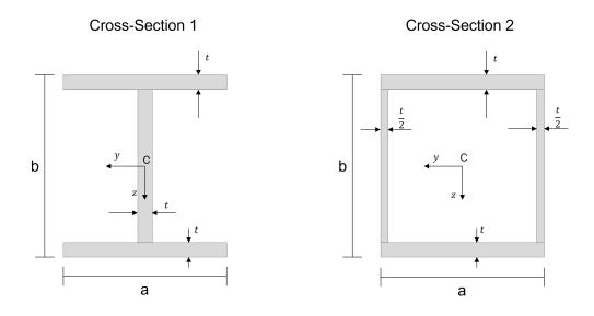
For the shown cross sections, which statement is true? ( $I_{yy}$  and  $I_{zz}$  are second moment of areas about the respective axis and  $I_T$  is the torsion constant of the cross-section)
