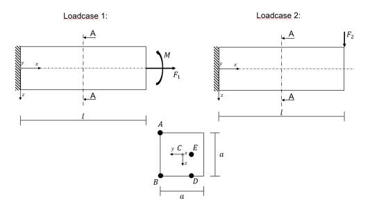
The shown clamped beam of length *I* is subjected to the moment *M* about the *y*-axis and the normal force  $F_1$  at it's free end in loadcase 1 and to the force  $F_2$  in loadcase 2. The cross-section and the modulus of elasticity are constant along the beam's x-axis. Each subtask is referring to only one of both loadcases. Use the given coordinate system with its origin in the cross sections centroid *C*.
