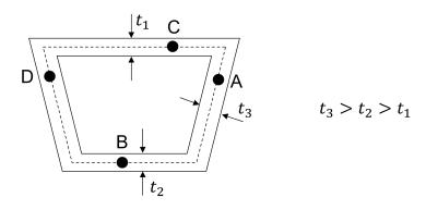
Shown is the thin-walled cross section of a bar. The bar is loaded by a torsional moment. At which point would one expect the greatest magnitude of the torsional shear stress  $|\tau|$ ?
