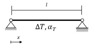
The shown bar is heated uniformly by  $\Delta T$ . The thermal expansion coefficient is constant ( $\alpha_T$ ). No other loads are applied. The displacement function u(x) will be:
