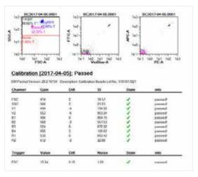
7 Successful calibration for each channel is indicated by a green check mark. When the process is successfully completed, the MACSQuant Instrument Status bar reports Acquisition Mode: Calibration OK. All settings will be automatically saved as default settings.
