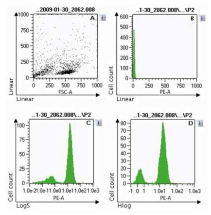
**Figure 2.9**: Comparing log and linear scales when displaying fluorescence intensities of fluorochrome-conjugated antibody binding. (A) Light scatter dot plot in linear scale. (B) PE fluorescence intensity in log5 scale. (D) PE fluorescence intensity in Hlog scale.
