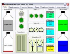
**Figure 11.1**: Example: Real-time Hardware monitor of the MACSQuant 10 Analyzer fluidic components.
