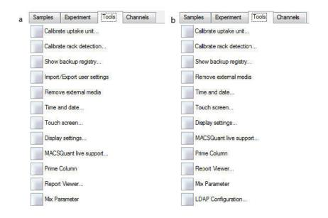
Figure 1.7: Tools available for administrators. Functions available for standard setup (a) or for CFR21 Part 11 compliant setup (b, refer to 21 CFR Part 11 compliance on page 165 for details).
