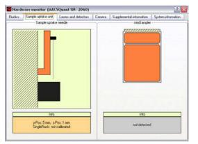
Figure 11.2: Example: Real-time hardware monitor of the MACSQuant 10 Analyzer sample uptake arm.
