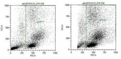
**Figure 2.7**: Trigger to exclude debris. Left: Debris represents 77% of sample. Right: After setting a trigger, debris represents 15% of sample.
