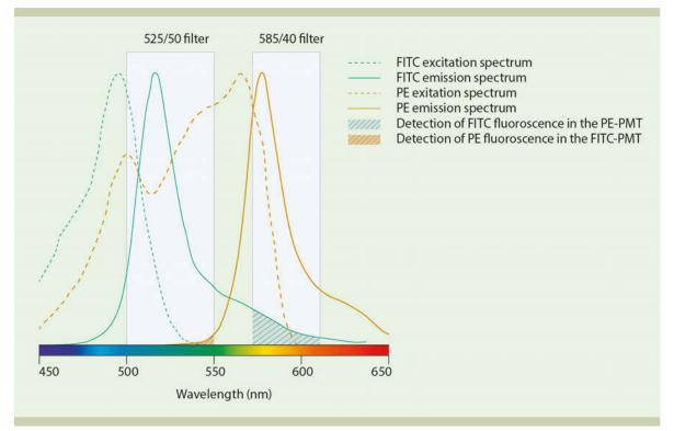
Figure 2.2: Emission spectra of FITC (green solid line) and PE (red solid line). The green hashed area represents the amount of FITC signal detected in B2. The red-hashed area represents the amount of PE signal detected in B1.
