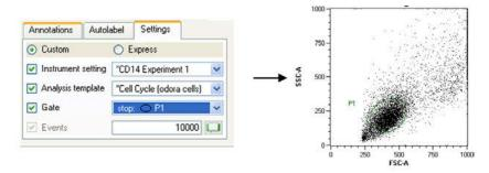
**Figure 4.4**: Region P1 is defined as a stop gate. At 1000 events, data acquisition stops automatically.
