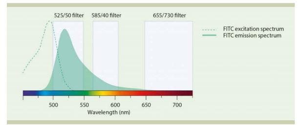
**Figure 2.5**: Spectrum of FITC single-stained cells. Green area: B1 (525/50) channel; yellow area: B2 (585/40) channel, red area: B3 (655–730) channel. In this example, 15% of the detectable FITC signal is seen in the B2 (PE) channel. To compensate, add 0.150 to the FITC-B2 box of the compensation matrix, and adjust the FITC-B1 box from 1.000 to 0.850. If additional spillover of the FITC signal is found in the B3 (PE-Cy5) channel, adjust values accordingly in box FITC-B3.
