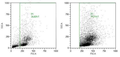
**Figure 2.1**: Adjustment of FSC and SSC PMT gains appropriate for PBMCs. Left: PBMCs prior to adjustment. Right: PBMCs after adjustment. A trigger has been set to exclude the debris.
