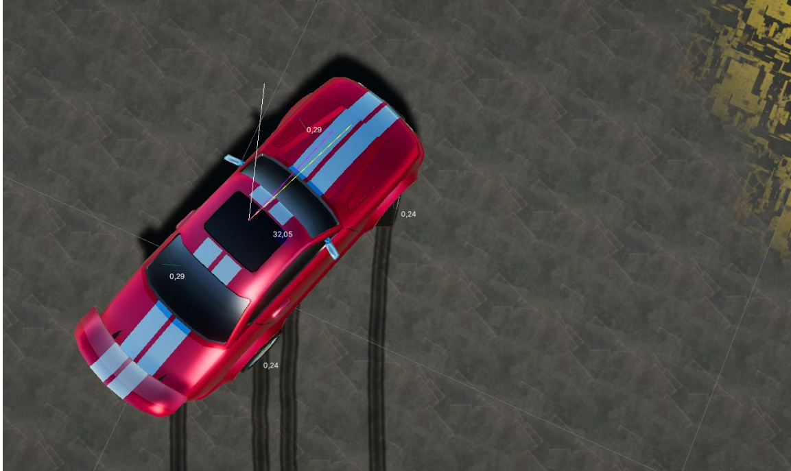
Drift Debug View. The white line displays the current direction of movement, the yellow line the drift target angle (determined by player input and the vehicle's drift parameters) and the pink line the vehicle's current forward vector.
