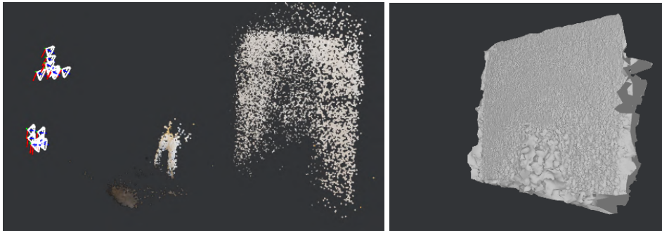
Figure 2.2: Structure from Motion with estimated camera locations, point cloud, and resulting mesh
