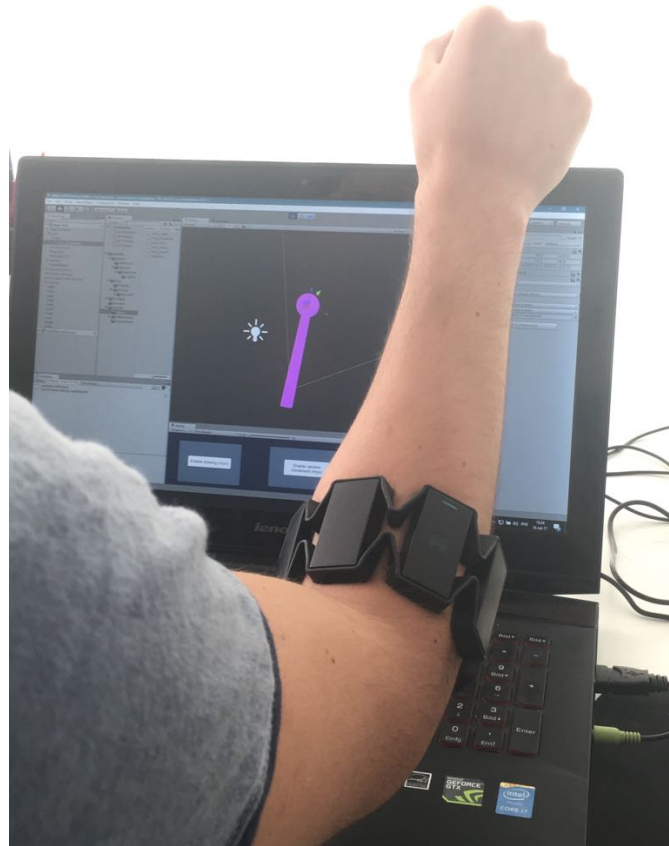
Figure 4.5: The arm and the joint GameObject are in sync after the updated reference.
