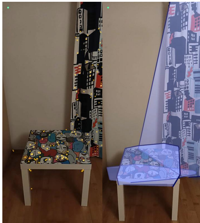
Fig 7-8. Left: Point Clouds; Right: Plane Detection
