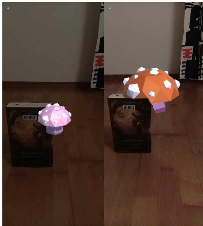
Fig 9-10. Left: No occlusion; Right: AR Occlusion Manager
