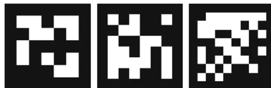
Figure 2.4: Examples of markers of different sizes, n , generated with the proposed method. From left to right: n=5 , n=6 and n=8 ; taken from [Gar+14], Figure 3
