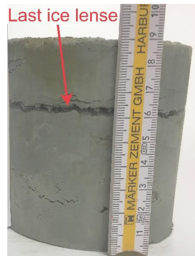
Fig. 2: Ice lens formation observed after a freezing test at Zentrum Geotechnik
