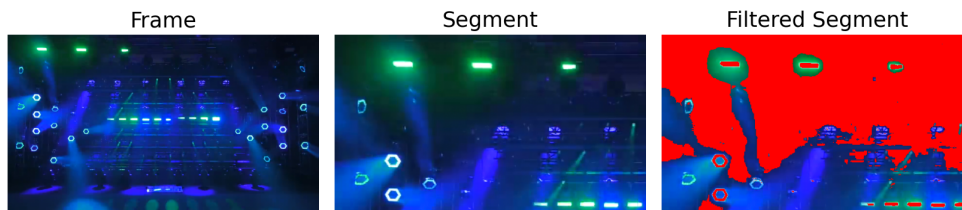
Figure 3.4: Splitting and filtering of a video frame
